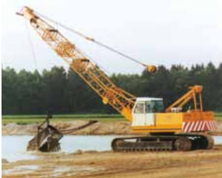
Milestone in the company history: The first fully hydraulic duty cycle crawler crane in the world launched in 1969.
