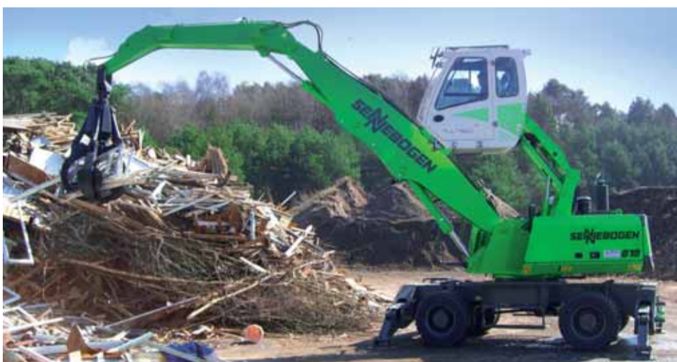
At GER Umweltschutz GmbH the SENNEBOGEN 818 is used to supply a wood shredder with 60 t wood per hour – often for 16 hours each day in two-shift operation.
