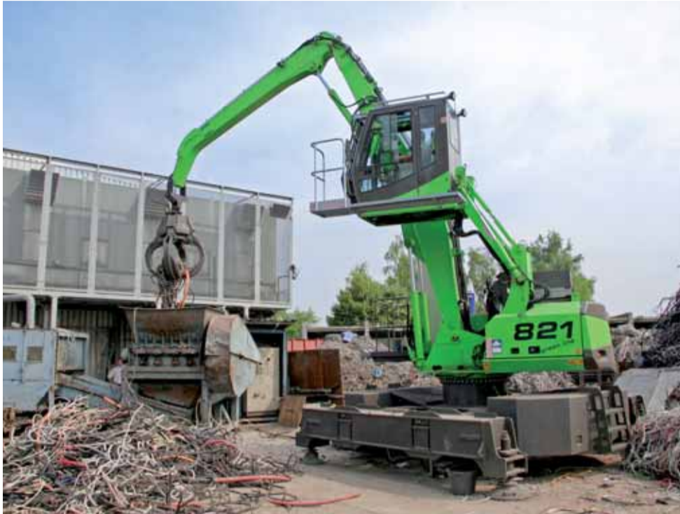
Quietly and powerful – up to 40 t of old cables are handled each day with the SENNEBOGEN 821 Electro.
