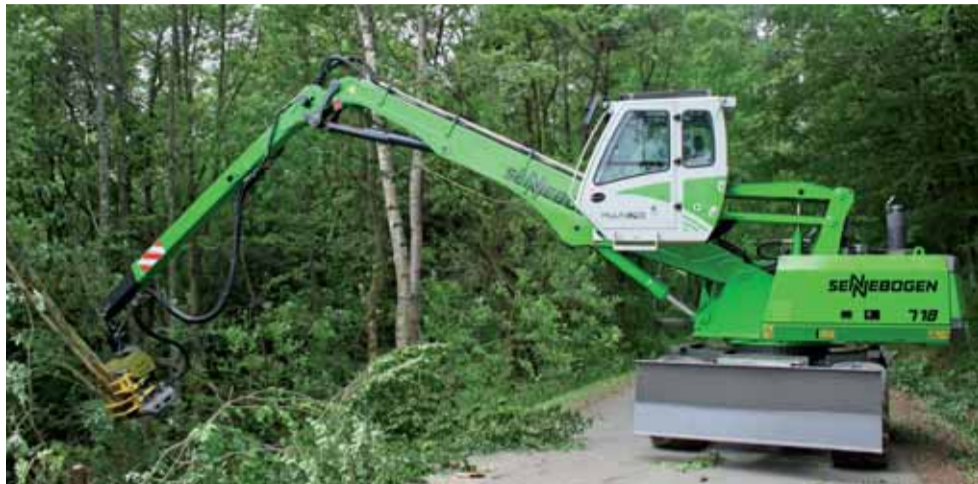
Very economical fuel wood harvest with the Bracke C16 felling head.
