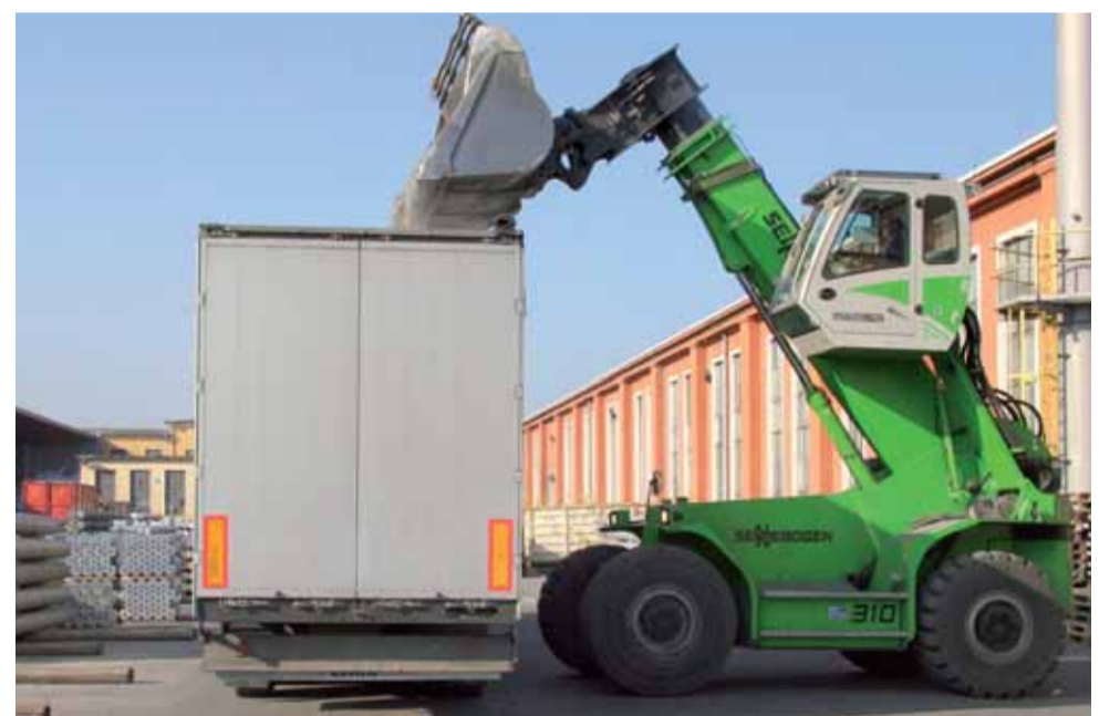
Convenient truck loading due to a cab that elevates to a viewing height of 5 m.
