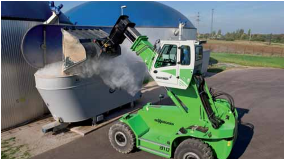
Superior view when filling the feeder thanks to the elevating cab.
