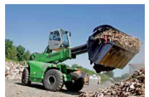
9.3 m lifting height and a max. load of 10 t – the SENNEBOGEN 310 Multiloader convinced in practical operation.
