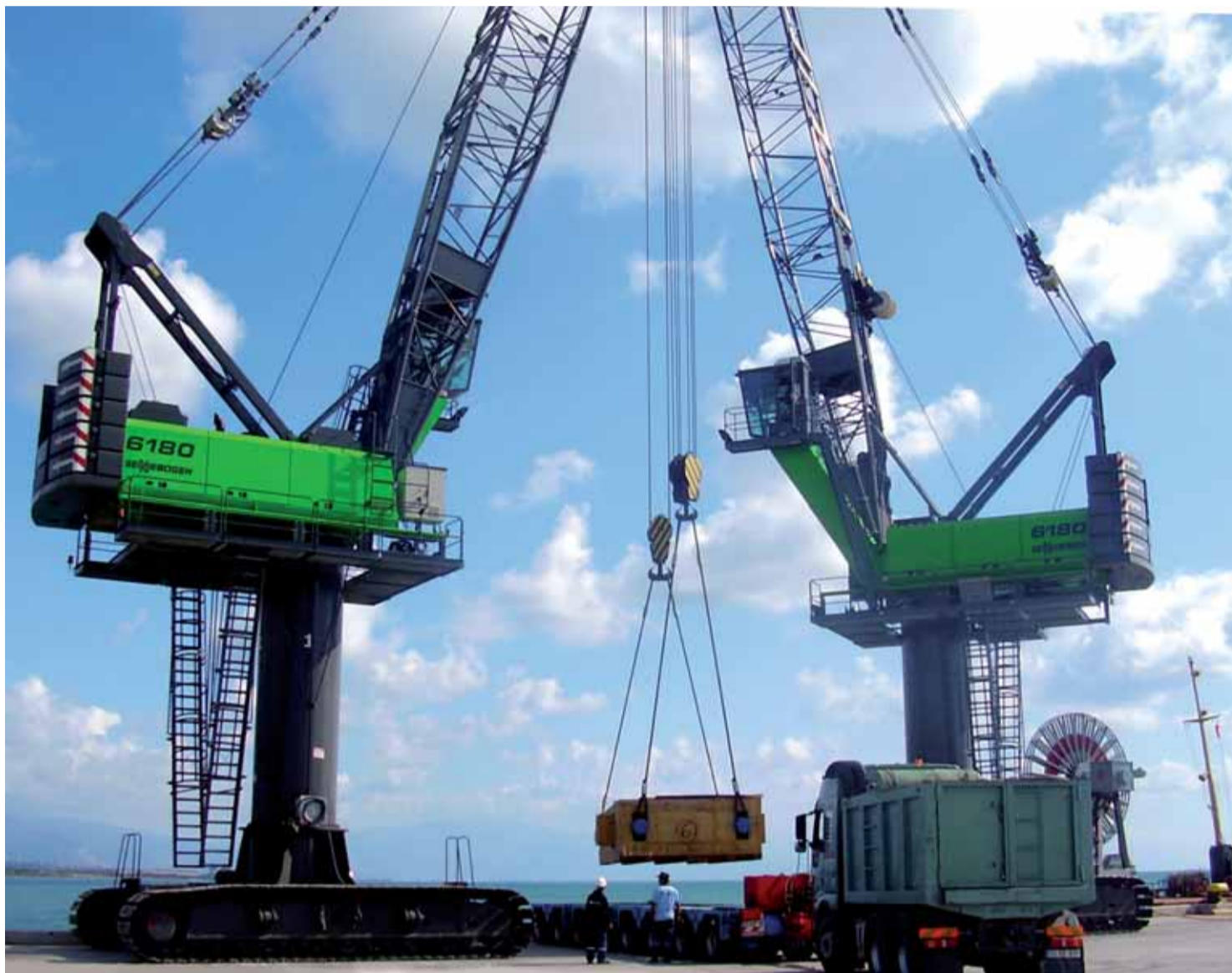
A total of eleven SENNEBOGEN machines with operating weights of up to 250 t are the green machine fleet at MMK-Atakas. Due to the modular structure the SENNEBOGEN machines can be adapted individually to the ship sizes and requirements on site. Each day not less than 14,000 t material from ships are unloaded and around 20,000 t are loaded.
