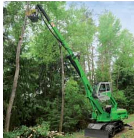
The SENNEBOGEN 718 offers a special boom system with 13 m reach and 1.6 t load.
