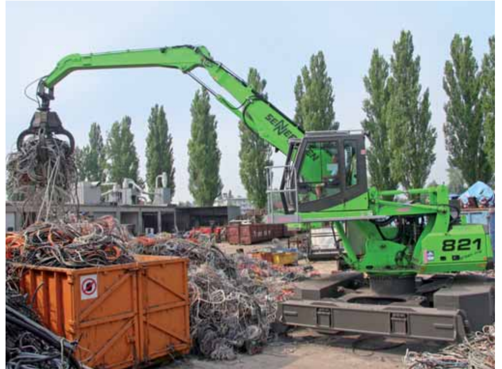
First step is sorting before shredding the around 10,000 t old cables a year at MVM München.
