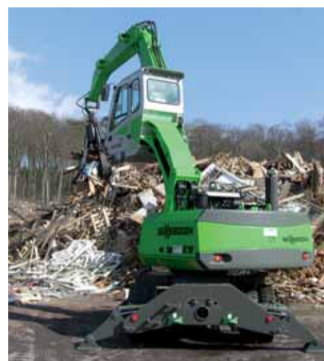
At GER Umweltschutz GmbH the SENNEBOGEN 818 is used to supply a wood shredder with 60 t wood per hour – often for 16 hours each day in two-shift operation.
