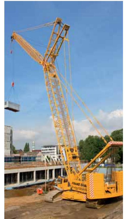
The new SENNEBOGEN 7700 with 300 t lifting capacity into use at the building site for the new Central Vocational College in Duisburg. The 29.9 m main boom and 41.1 m luffing jib creates the necessary large working radius of up to 60 m.
