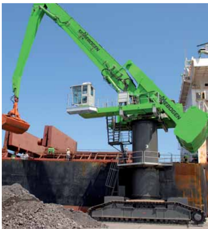
A total of eleven SENNEBOGEN machines with operating weights of up to 250 t are the green machine fleet at MMK-Atakas. Due to the modular structure the SENNEBOGEN machines can be adapted individually to the ship sizes and requirements on site. Each day not less than 14,000 t material from ships are unloaded and around 20,000 t are loaded.
