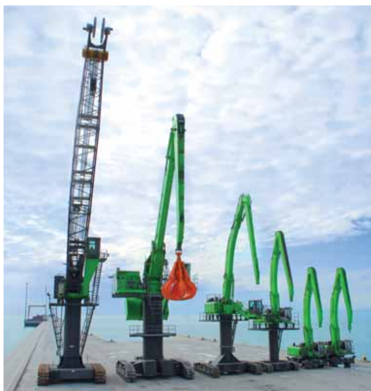
A total of eleven SENNEBOGEN machines with operating weights of up to 250 t are the green machine fleet at MMK-Atakas. Due to the modular structure the SENNEBOGEN machines can be adapted individually to the ship sizes and requirements on site. Each day not less than 14,000 t material from ships are unloaded and around 20,000 t are loaded.
